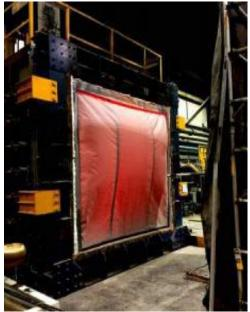
Kent Automatic Fire Curtains are life safety systems that are designed to arrest the spread of fire in a building. The assembly comprises a fire resistant fiberglass fabric wound over a roller and all encased in a compact head box that is typically installed above the ceiling to be virtually invisible until activated.
